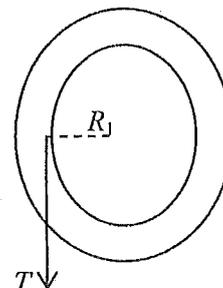
$$\sum M = I_T \gamma \xrightarrow{\text{reemplazo}} +T \cdot R_1 = 3,24 \cdot 10^{-3} \text{ kg} \cdot \text{m}^2 \cdot \gamma$$
