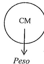
$$\sum_{=0} M = I_{cm} \cdot \gamma \rightarrow \gamma = 0 \rightarrow \omega = 5\text{ s}^{-1} = \text{cte}$$
